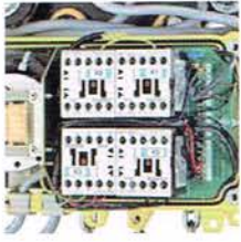
Increased operating safety through 42 V control voltage
